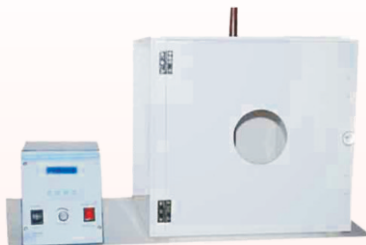
SMC 90144 POLE CLIMBING APPARATUS (COOK'S) Outer chamber made of thick plywood with observation window & inner made of clear acrylic sheet, with chrome plated brass bars at bottom. A shock for controlled duration of 200V AC 50Hz single phase 0.2 Ma is built in & controlled by solid state timer.
