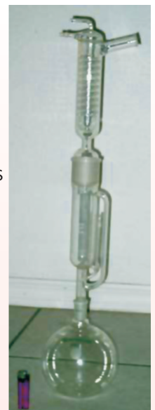
SMC 90148 SOXHLET EXTRACTION APPARATUS (Borosilicate Glass) SMC 90148/1 Capacity 100ml SMC 90148/2 Capacity 200ml SMC 90148/3 Capacity 500ml
